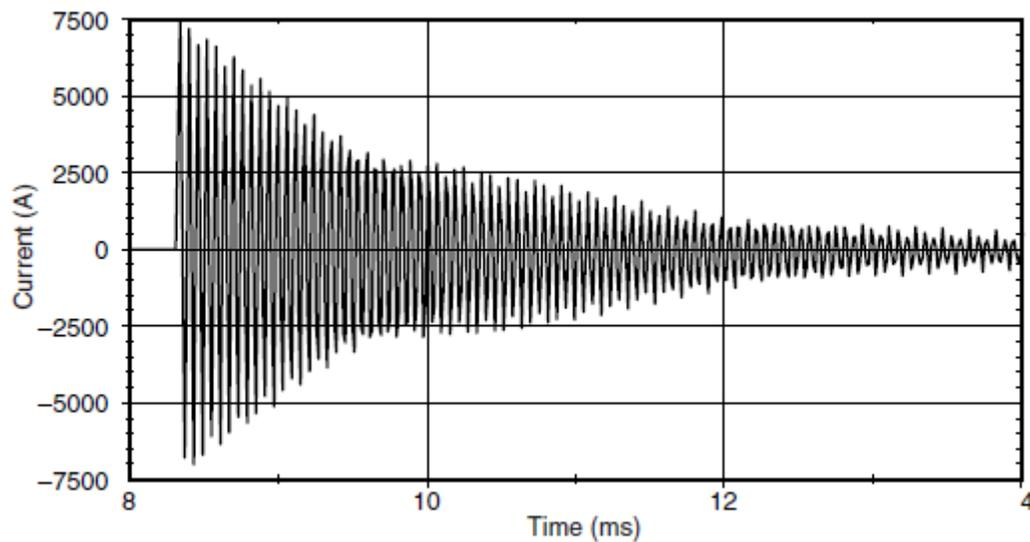
**Figure 3.1** Oscillatory transient current caused by back-to-back capacitor switching
