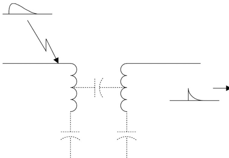
**Figure 3.4** Coupling of impulses through the inter-winding capacitance of transformers
