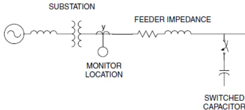
**Figure.3.2** capacitor Switching
