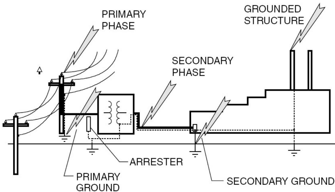
**Figure 3.3** Lightning strike locations where lightning impulses will be conducted into load facilities
