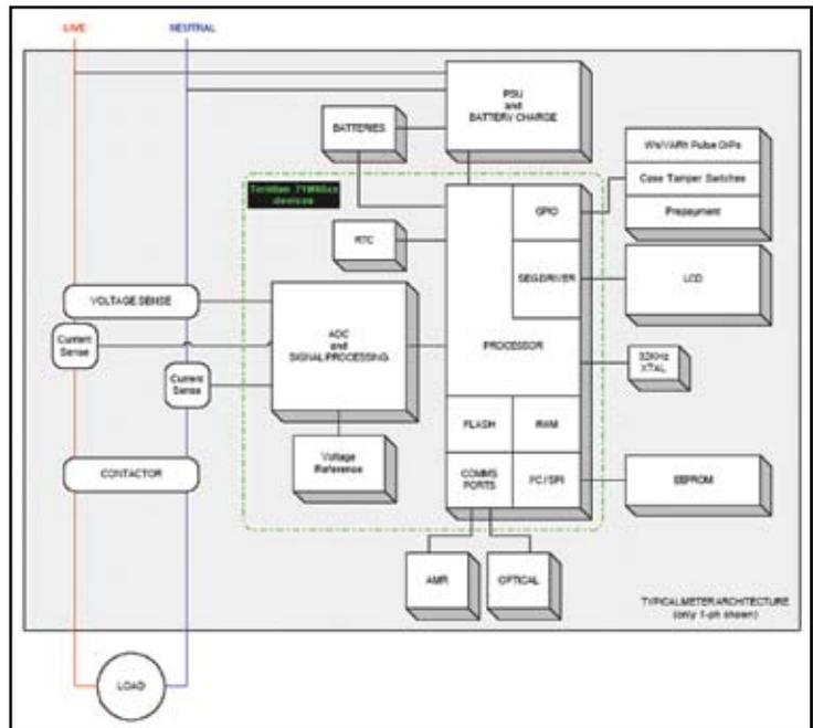
Figure 3 – Typical meter architecture
