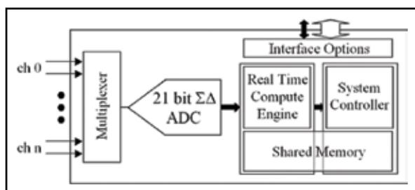
Figure 2 – Division of functionality in a mixed signal metrology subsystem
