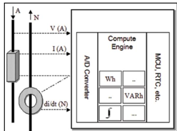
Figure 1 – The highly integrated 71M6521 metering IC with single converter technology
