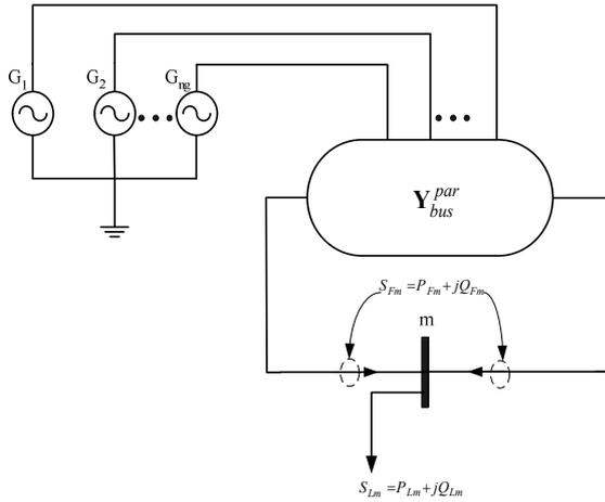
**Fig.2.** The complex power balance of bus m
