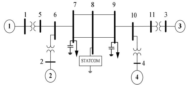
**Fig.8.** Single line diagram of Kundur’s inter-area power system equipped with a STATCOM
