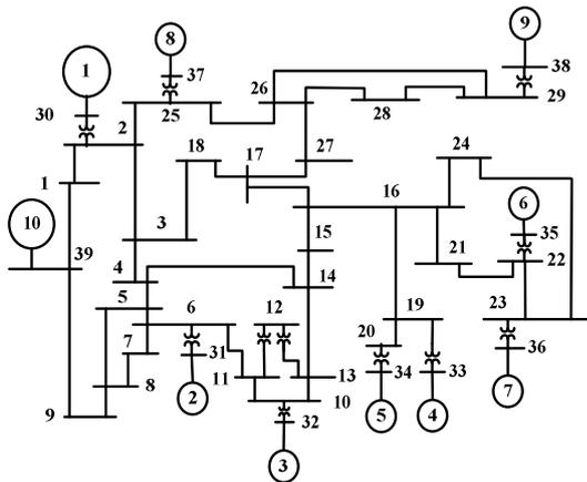
**Fig.10.** Single line diagram of new England system equipped with a STATCOM
