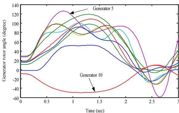
**Fig.11.** Generator rotor angle of new England system without STATCOM for  $t_{cl}$ =190 msec
