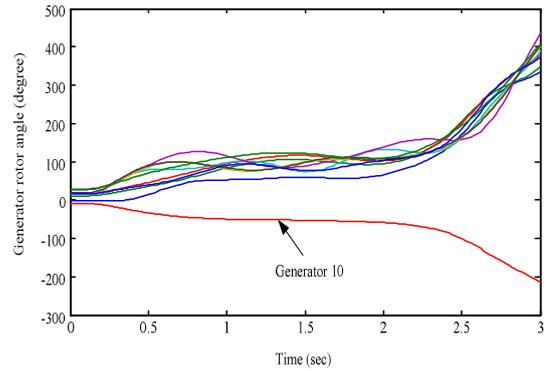
**Fig.12.** Generator rotor angle of new England system without STATCOM for  $t_{cl}$ =191 msec
