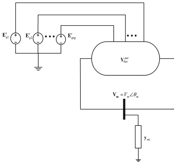
**Fig.7.** Equivalent circuit of multimachine power system equipped with a STATCOM represented by susceptance  $y_{mi}$
