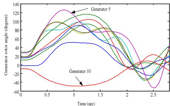
**Fig.13.** Generator rotor angle of new England system with a STATCOM for  $t_{cl}$ =191 msec
