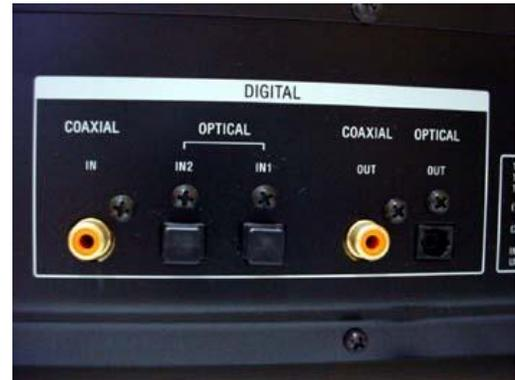
**Figure 6:** Rear of a Mini Disc deck, you can see from left to right one coaxial SPDIF input, two optical SPDIF inputs, one coaxial SPDIF output and one optical SPDIF output.
