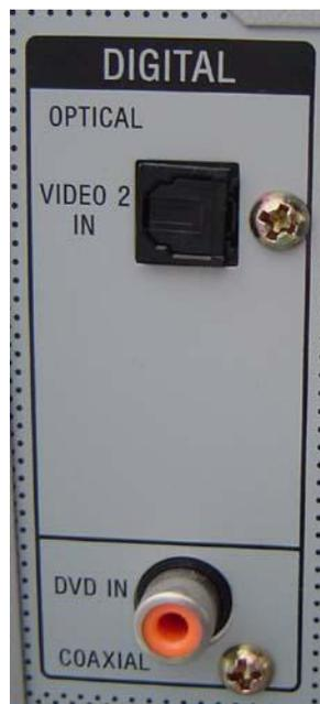
**Figure 9:** Optical and coaxial SPDIF inputs on a
