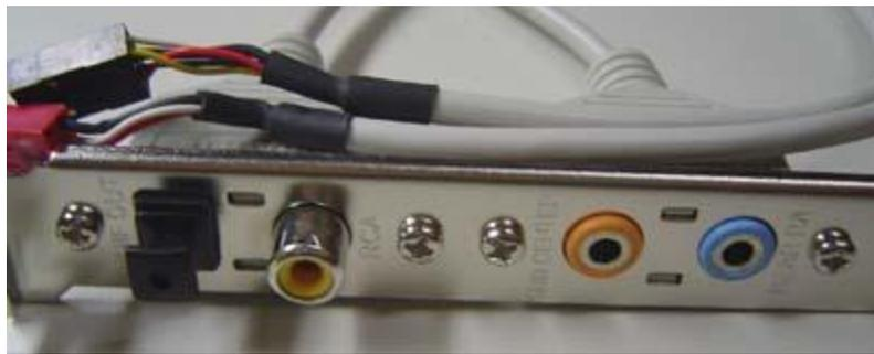
**Figure 12:** SPDIF adaptor from Gigabyte K8NXP motherboard has only outputs (both optical and coaxial).
