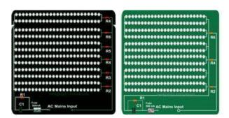
Referring to the figure, a glance shows it to be a rather standard configuration where a capacitive current dropped power supply is incorporated to drive some groups of LEDs. However a careful investigation reveals that the circuit does not include a bridge and a capacitor network, usually employed with power supplys, especially for driving LEDs.
