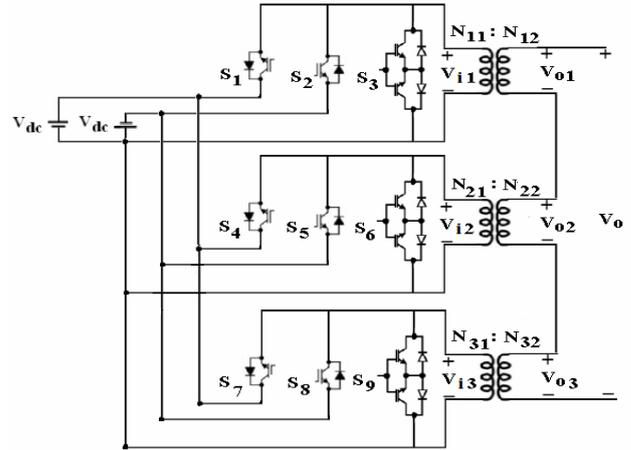
**Fig. 4.** Proposed topology with three basic units.
