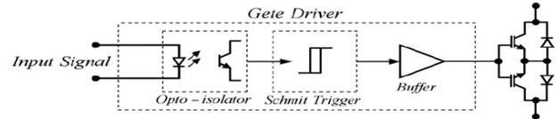
Fig. 3. Bi-directional switch and one type gate driver circuit.
