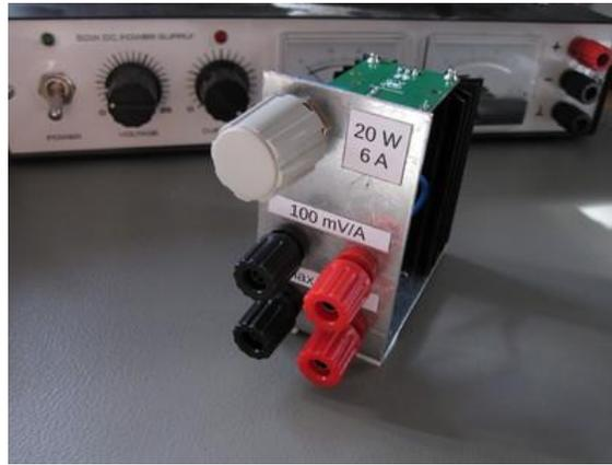
I connected the load and the current sense wires to terminals on the front panel. I also found a matching  $10\text{ k}\Omega$  potentiometer with a knob for setting the current.
