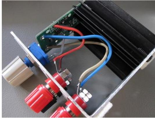
As far as I have tested it, Re:load 2 seems to work as advertised. I haven't noticed any drift in current I could notice with my multimeter when Re:load is heating up. I did notice though that with the 6 A range it gets hard to set currents below 1 A even with the large knob I added. A fine-adjustment pot might be handy in those cases.
