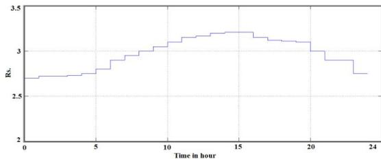
Figure 8. Real Time Pricing signal
