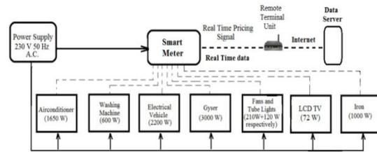
Figure 5. Block diagram of Home Area Network
