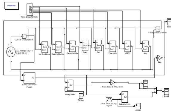
Figure 6 Simulink Model of Home Area Network.
