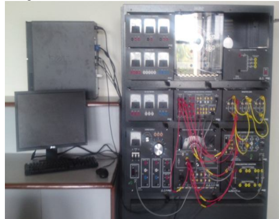
Figure 4: Experimental setup of buck converter.
