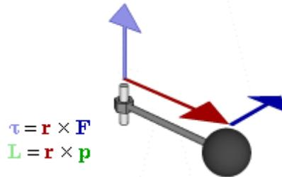
Relationship between Force  $\mathbf{F}$ , torque  $\tau$ , linear momentum  $\mathbf{p}$ , and Angular momentum  $\mathbf{L}$  in a system which has rotation constrained in one plane only (forces and moments due to gravity and Friction not considered).
