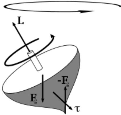
The torque caused by the two opposing forces  $F_g$  and  $-F_g$  causes a change in the angular momentum  $L$  in the direction of that torque. This causes the top to precess.
