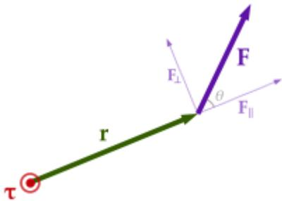
A particle is located at position  $\mathbf{r}$  relative to its axis of rotation. When a force  $\mathbf{F}$  is applied to the particle, only the perpendicular component  $\mathbf{F}_\perp$  produces a torque. This torque  $\boldsymbol{\tau} = \mathbf{r} \times \mathbf{F}$  has magnitude  $\tau = |\mathbf{r}| |\mathbf{F}_\perp| = |\mathbf{r}| |\mathbf{F}| \sin\theta$  and is directed outward from the page.
