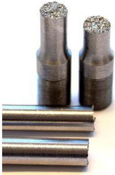
This tensile test of a nodular cast iron demonstrates low ductility.
