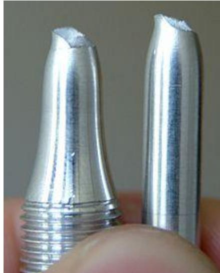
Tensile test of an AlMgSi alloy. The local necking and the cup and cone fracture surfaces are typical for ductile metals.
