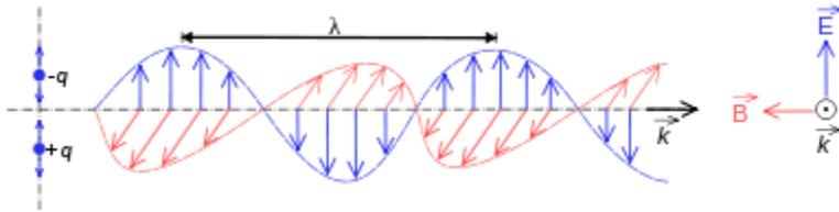
The electromagnetic waves that compose electromagnetic radiation can be imagined as a self-propagating transverse oscillating wave of electric and magnetic fields. This diagram shows a plane linearly polarized EMR wave propagating from left to right. The electric field is in a vertical plane and the magnetic field in a horizontal plane. The two types of fields in EMR waves are always in phase with each other with a fixed ratio of electric to magnetic field intensity.
