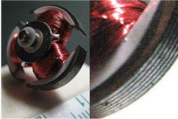
This is a rotor approximately 20mm in diameter from a DC motor used in a CD player. Note the laminations of the electromagnet pole pieces, used to limit parasitic inductive losses.
