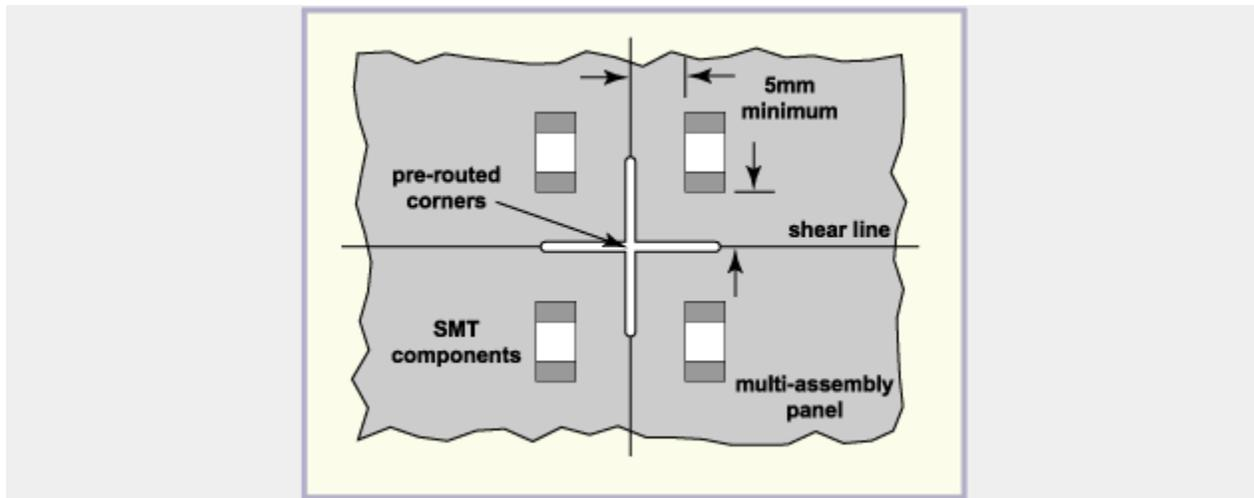
**Figure 2: Guidelines for positioning MLCs for minimum stress**
