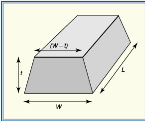
Figure 1: Trapezoidal cross-section of a track on a PCB
