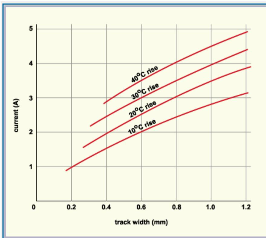
Figure 2: Heat rise in a 70  $\mu\text{m}$  copper foil as a function of current and track width
