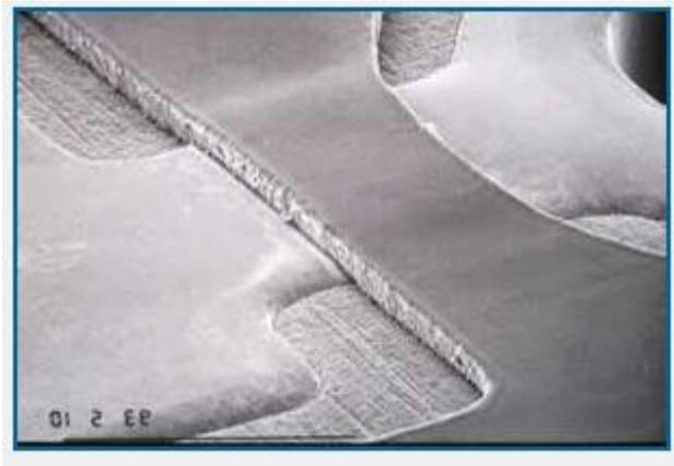
Figure 1: Example of dry film resist side walls
