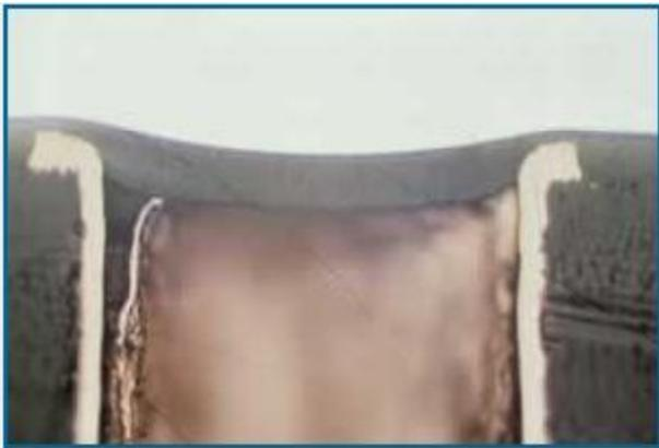
Figure 4: A via tented with dry film resist
