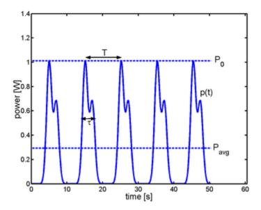
In a train of identical pulses, the instantaneous power is a periodic function of time. The ratio of the pulse duration to the period is equal to the ratio of the average power to the peak power. It is also called the duty cycle (see text for definitions).
