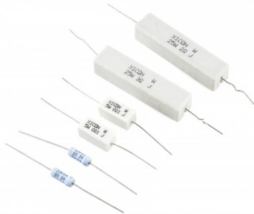
*These power resistors can handle a lot more power before they blow. From top-right to bottom-left there are examples of 25W, 5W and 3W resistors, with values of 2Ω, 3Ω 0.1Ω and 22kΩ. Smaller power-resistors are often used to sense current.*
