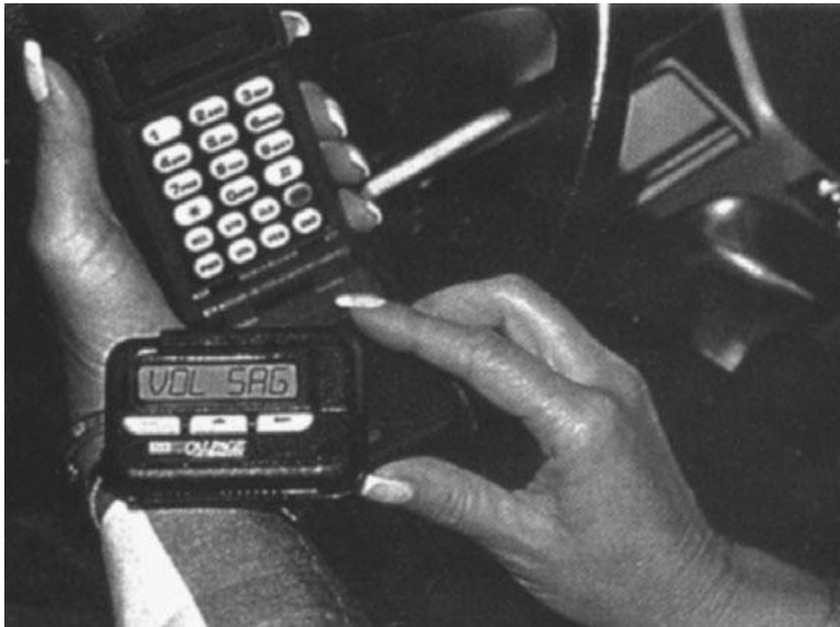
Figure 5.7 Power quality pager
