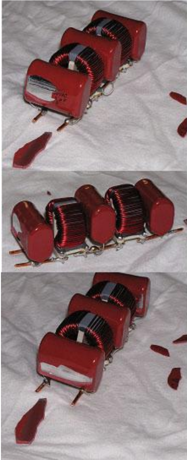
Figure 6. Example EMI filter from resonant overvoltage during surge test: line-side of filter showing damaged X-capacitor (top); side view of filter showing no damage to center X-capacitor (middle); load-side of filter showing damaged X-capacitor (bottom).
