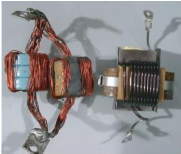
Figure 9. Two inductors from power-line filters - (left) saturates at a low current while (right) does not saturate at specified filter load current.
