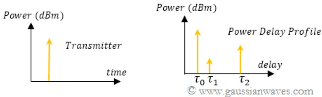
Power Delay Profile is usually supplied as a table of values obtained from empirical data and it serves as a guidance to system design. Nevertheless, it is not an accurate representation of the real environment in which the mobile is destined to operate at.
