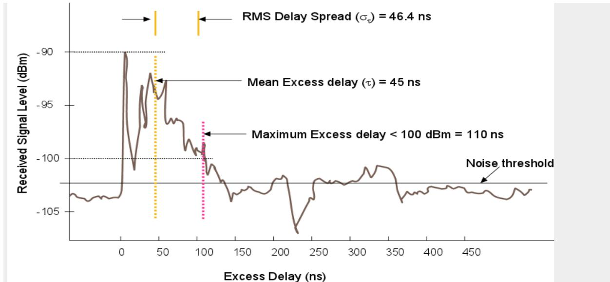
Power Delay Profile with Mean delay, RMS delay spread, Maximum Excess Delay
