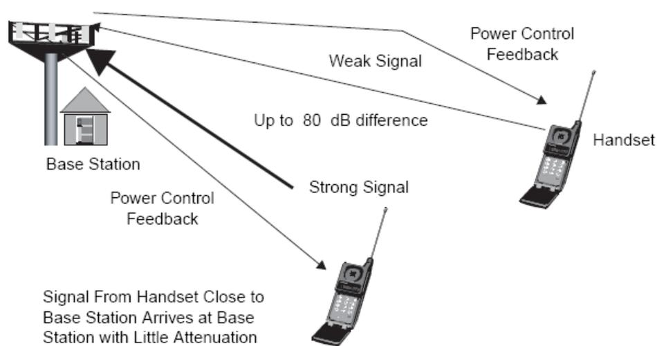
**Figure 11.19 Power control in CDMA.**
