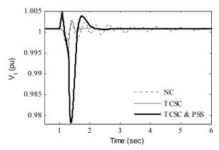
Fig. 14 Variation of terminal voltage  $V_t$ : Case-1
