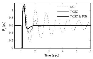
Fig. 10 Variation of electrical power  $P_e$ : Case-1
