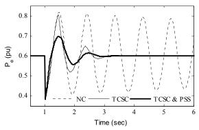
Fig. 20 Variation of electrical power  $P_e$ : Case-2
