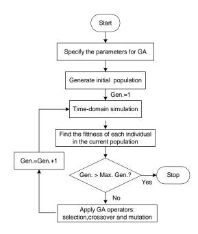
Fig. 4 Flowchart of the genetic algorithm
