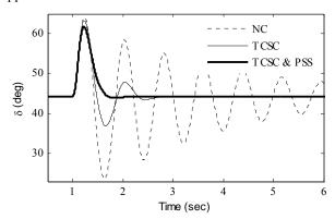
Fig. 8 Response of power angle  $\delta$  for a 5-cycle three-phase fault disturbance (Case-I)
