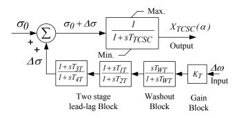
Fig. 2 Structure of TCSC-based controller
