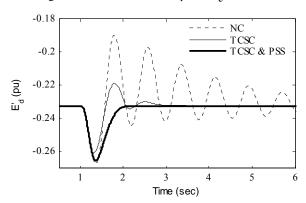
Fig. 11 Variation of voltage  $E'_{d}$ : Case-1
