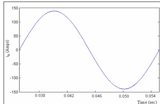
Fig. 7 (f) Phase A line current of SVM VSI with 1-9-9-3 network and  $T_s=50\mu s$
