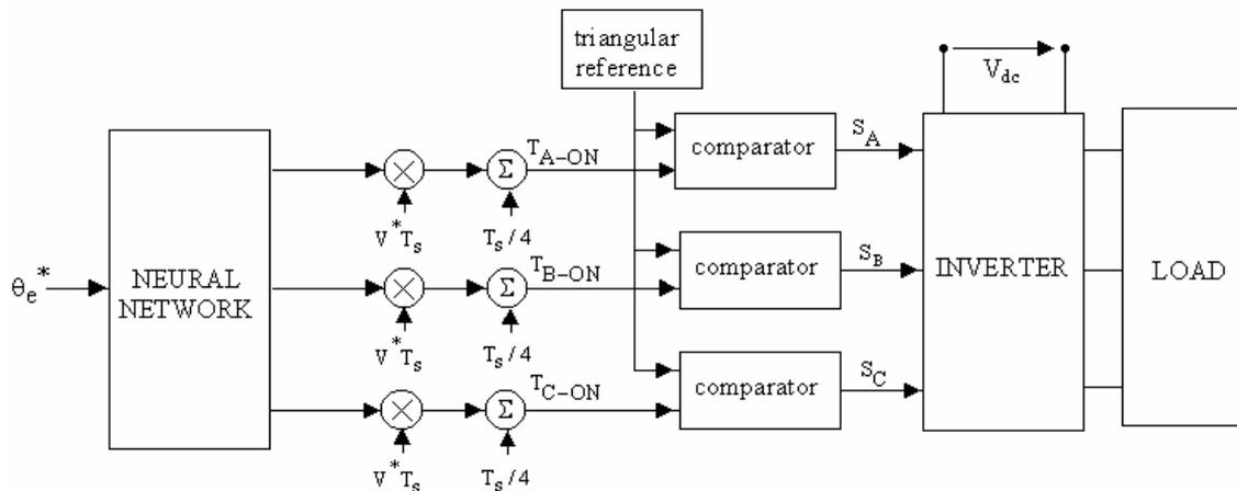
Fig. 6 Schematic of the ANN based SVM inverter
