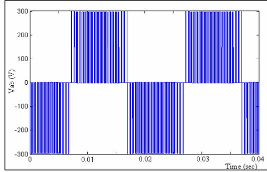
Fig. 7 (b) Line voltage ( $V_{ab}$ ) of SVM VSI with 1-9-9-3 network and  $T_s=500\mu s$
