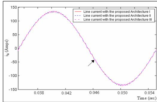
Fig 7 (d) Line current of phase A with proposed architectures for  $T_s=500\mu s$
