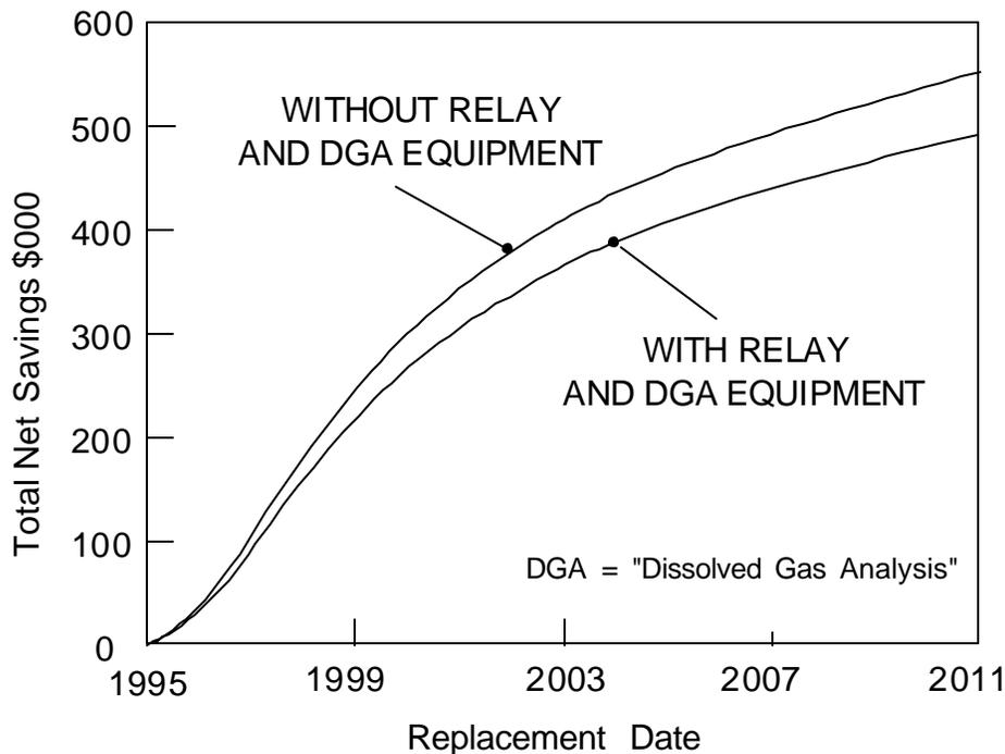
Fig. 6 - Total net savings in 1994 present value dollars. total net savings by delaying the replacement date of the new transformer from 1 to 16 years. In general the
