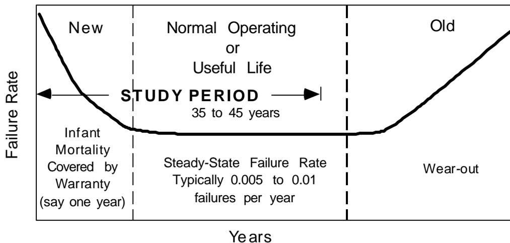
Fig. 5 - Typical failure rate curve.
