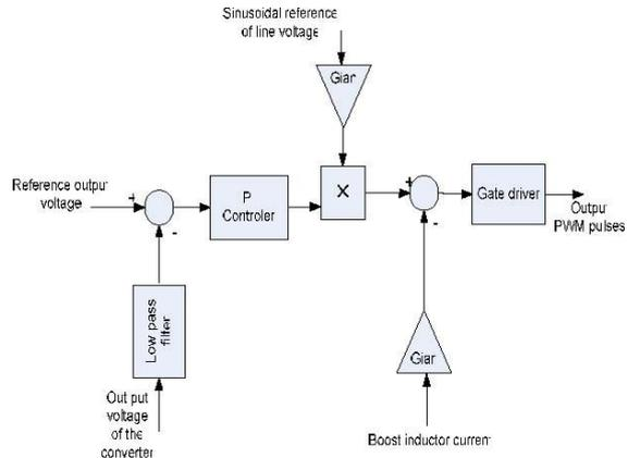
Figure.2 PWM controller with two feedback loops
