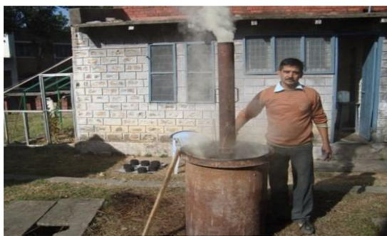
Fig1: Carbonizer drum
