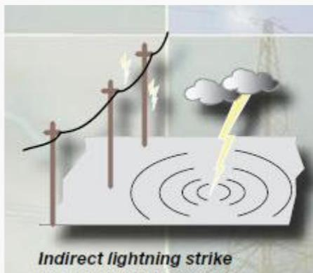
Left: Direct lightning strike on overhead line; Right: Indirect lightning strike on ground
