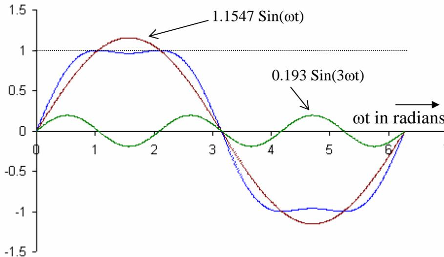
**Fig. 38.1: The modulating signal for Sine+3<sup>rd</sup> harmonic modulation**
