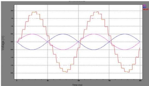
Fig. 12 Sample and Hold output at 100Mps
