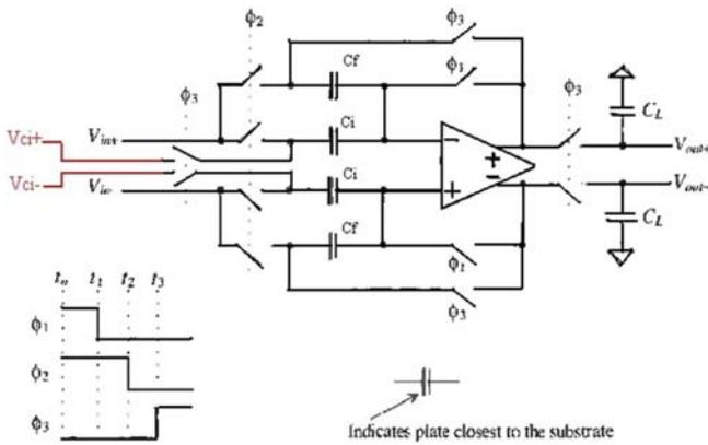
Fig. 11 Switched Capacitor Sample and Hold circuit
