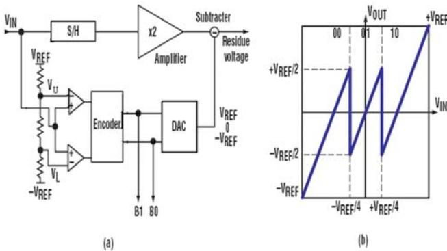
Fig.7 a) MDAC for 1.5 bit conversion b) transfer characteristic
