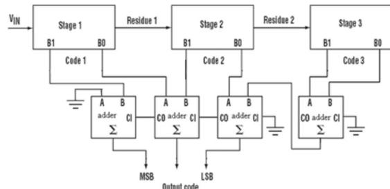
Fig. 8 Implementation of redundancy bit removal algorithm
