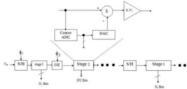
Fig. 5 Pipeline ADC Architecture
