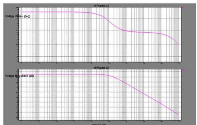
Fig. 10 Gain and phase margin of Op-amp
