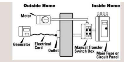
Manual transfer switch is the safest than automatic.
