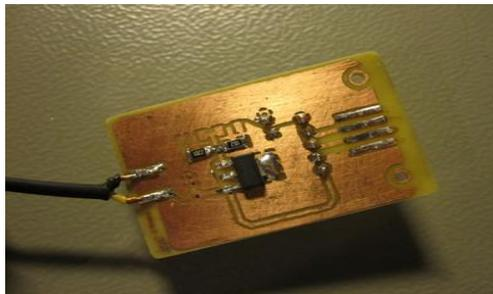
This led to me to make this tiny power adapter that attaches to the main PCB instead of the battery. It provides all the power for Kindle's main board which has another benefit of freeing up the USB connector for any future hacks (switching to USB host mode would be nice).
