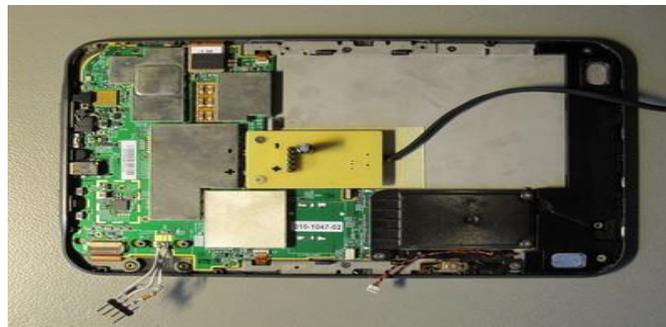
However, as many people on the web with dead Kindle batteries found out, Kindle won't boot with no voltage on the battery connector. Looking into the supply tree in the MC13892 datasheet it's apparent that the battery voltage is the central point from which all other parts are powered. The datasheet also explicitly states that the MC13892 will not power up the CPU unless it detects a valid voltage on the battery, even if power is available from the USB interface.
