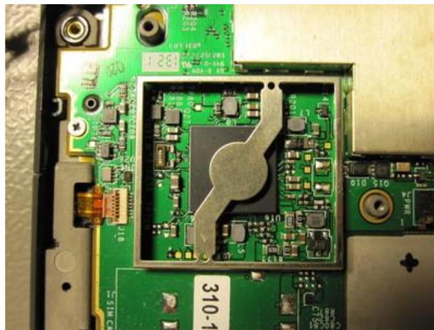
The chip itself hides under one of the shiny RF shielded enclosures and is connected to the main CPU over an SPI bus. The MC13892 datasheet reveals a very flexible chip that contains several configurable switching and linear power supplies, handles power on an USB bus and can work with a main and a backup battery. It also has peripherals like the real time clock, touch screen, temperature and light sensor interface and several programmable LED drivers.
