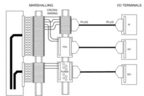
From a high level, cross-wire marshalling combines elements of the half-knit and fan-out marshalling schemes. Cross-wire marshalling takes field cables and terminates them in pair order. Scrambling is done to the disconnects, fuses, or termination assemblies. Common prefabricated cables are used between the disconnects and system cabinets.
