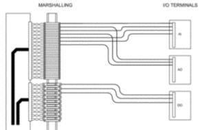
Half-knit marshalling performs the scrambling on the system side. The field cables are terminated on marshalling blocks in pair order, making this very efficient and easy to maintain. This type of marshalling arrangement is suitable in several situations:
