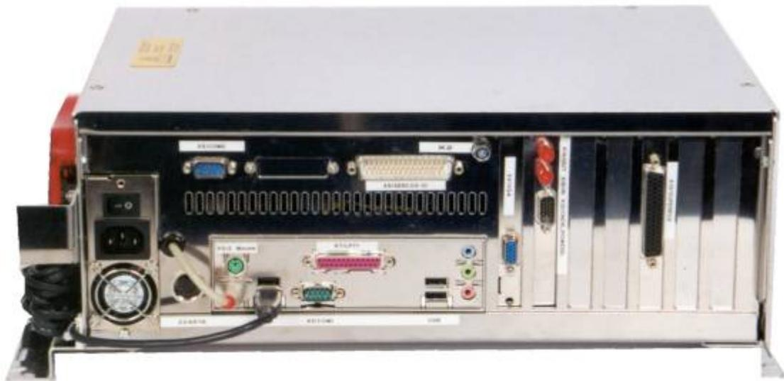
Figure 7. CE Rated Stainless Steel Industrial Personal Computer
