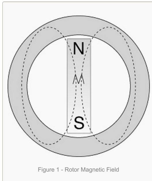
Figure 1 - Rotor Magnetic Field
