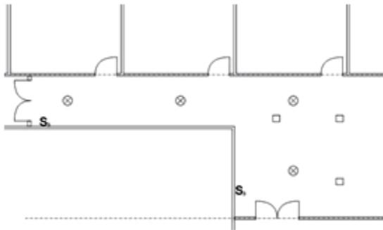
In the image to the left we can identify a hallway that goes into a larger common area and two double door exits. What multiway switching does, is to allow us to control the 4 lights in this area from either one of these exits by connecting a 3 **way switch** near the doors.
