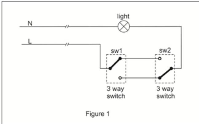
As depicted in figure 1 the light is off and in figure 2 we turn on the light with sw1 in 2.a and with sw2 in 2.b.
