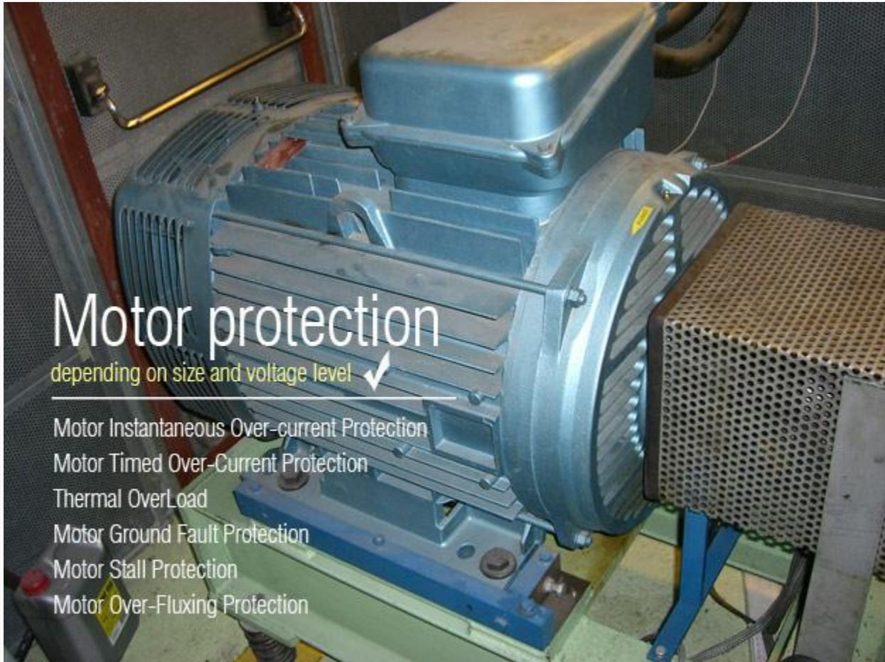
*Motor protection depending on size and voltage level (on photo 3-phase asynchronous motor LeroySomer P280 S-8, 55 kW)*
