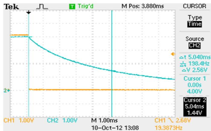
Murata capacitors yielded 5.1  $\mu$ F using the RC method, Multicomp capacitors yielded 3.9  $\mu$ F.
