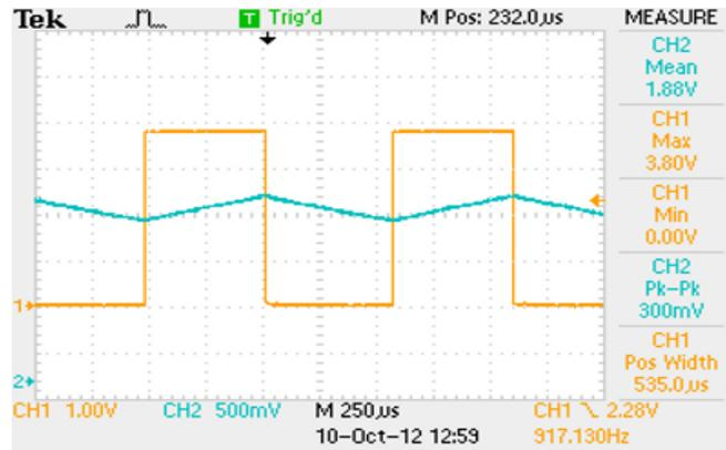
Murata capacitors yielded 3.5  $\mu$ F using the  $dU/dt$  method, Multicomp capacitors yielded 3.3  $\mu$ F.
