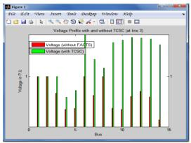
Fig 7: Voltage profile with and without TCSC (at weakest bus 3)
