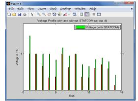
Fig 5: Voltage profile with and without STATCOM (in weakest bus 4)
