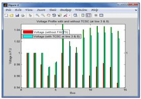
Fig 8: Voltage profile with and without TCSC at weakest bus 3 and weak bus 8
