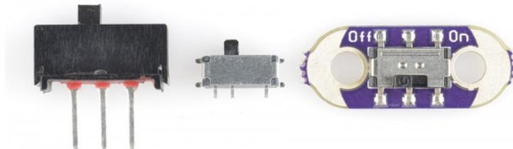
*Some examples of slide switches: a mini PTH slide switch, an SMD right-angle switch, and an SMD DPDT slide switch mounted on a LilyPad.*
