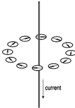
**Figure o:** The magnetic field curls around the wire in circles. At each point in space, the magnetic compass shows the direction of the field.
