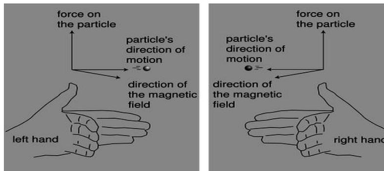
**Figure q:** The force on a charged particle moving through a magnetic field is perpendicular to both the field and its direction of motion. The relationship is right-handed for one type of charge, and left-handed for the other type.
