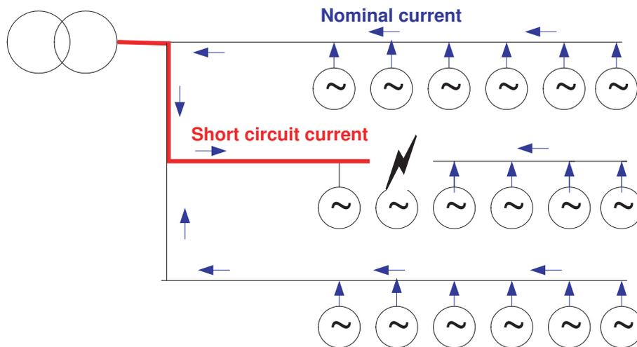
Figure 5: Nominal and short circuit current flows after fault
