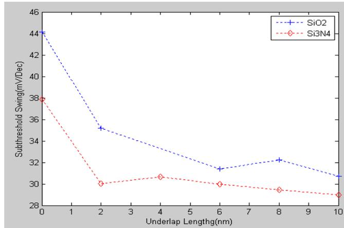
Fig 3: Effect of variation of underlap length on Subthreshold swing(S)
