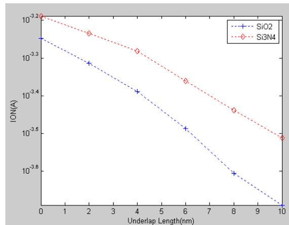
Fig7: Effect of variation of underlap length on  $I_{ON}$
