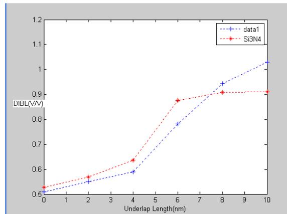
Fig 6:Effect of variation of underlap length on DIBL
