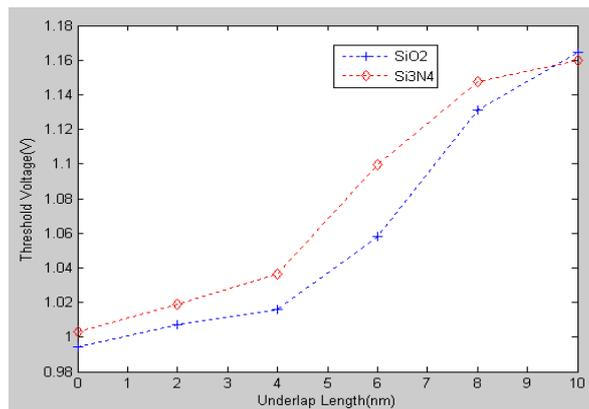
Fig4: Effect of underlap in BOI FinFET on threshold voltage (Vth)
