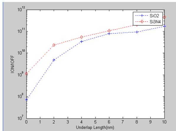
Fig8: Effect of variation of underlap length on  $I_{ON}/I_{OFF}$
