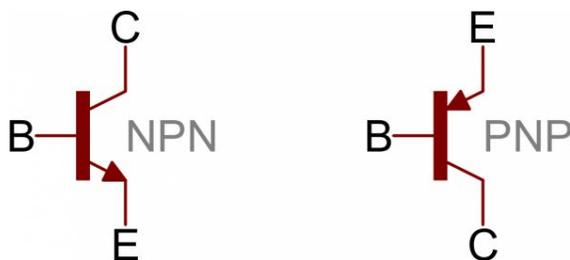
The only difference between an NPN and PNP is the direction of the arrow on the emitter. The arrow on an NPN points out, and on the PNP it points in. A useful mnemonic for remembering which is which is:
