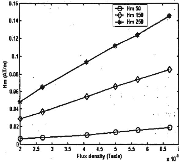
Fig. 5. B-Hm curve of core at 50, 150 and 250 Hz magnetization.
