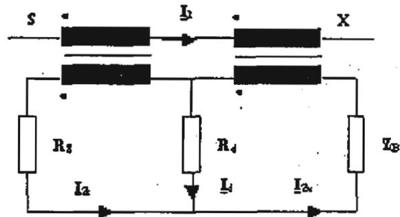
Fig. 3. The Comparison method of testing a CT
