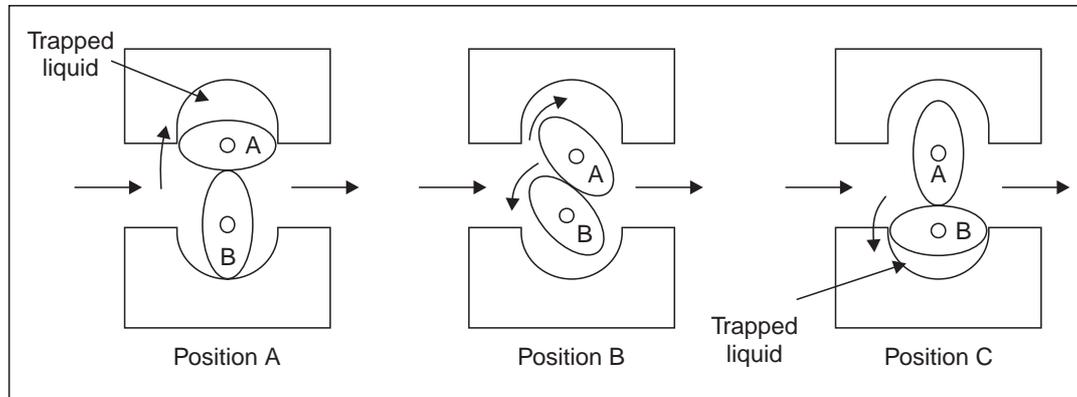
**Fig. 1.31** Working principle of Oval-gear flow meter
