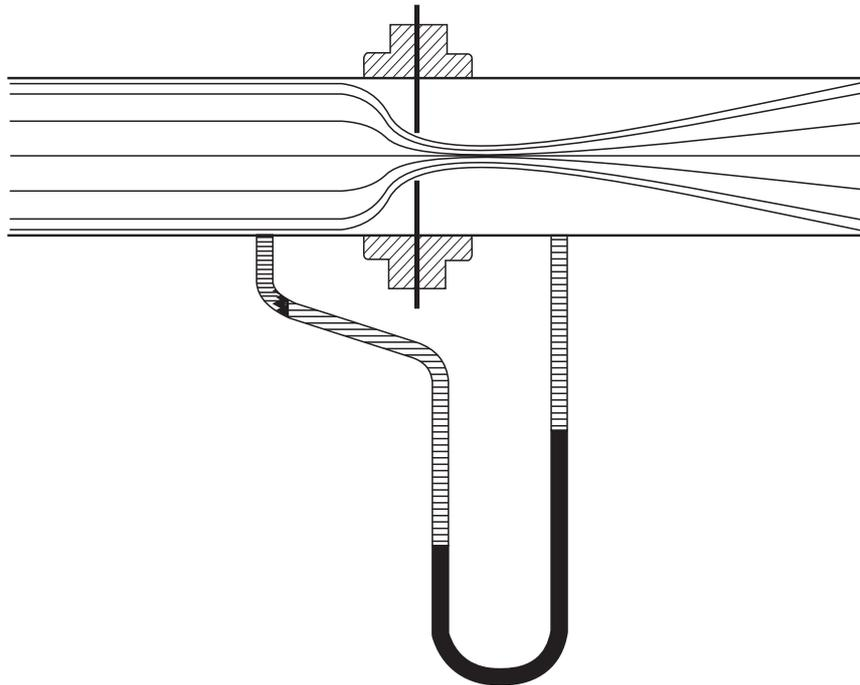
**Fig. 1.2** Orifice and Pressure-Differential Measurement
