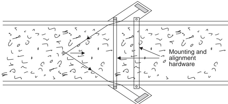
**Fig. 1.60** Two-transducer approach
