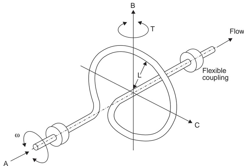
Fig. 1.42 Gyroscopic Mass Flow meter
