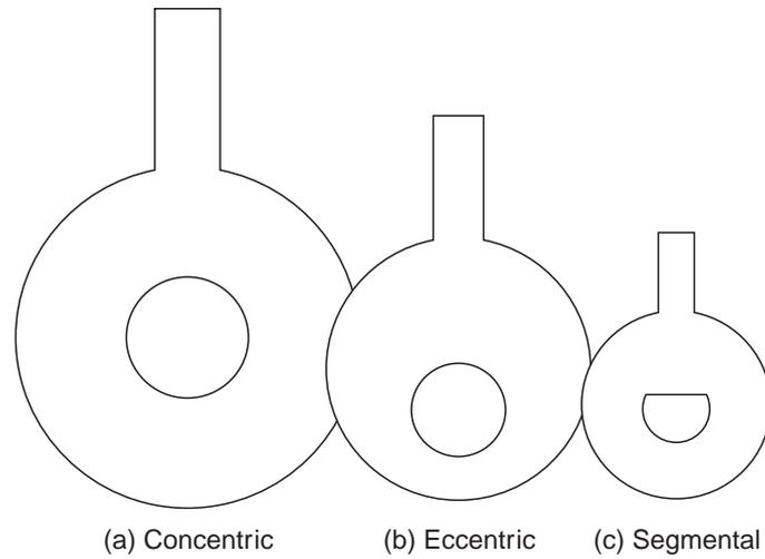
**Fig. 1.4** Sketch of orifices of different types
