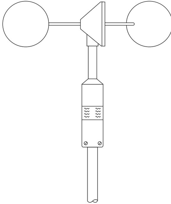
**Fig. 1.81** Three cup-anemometer.
