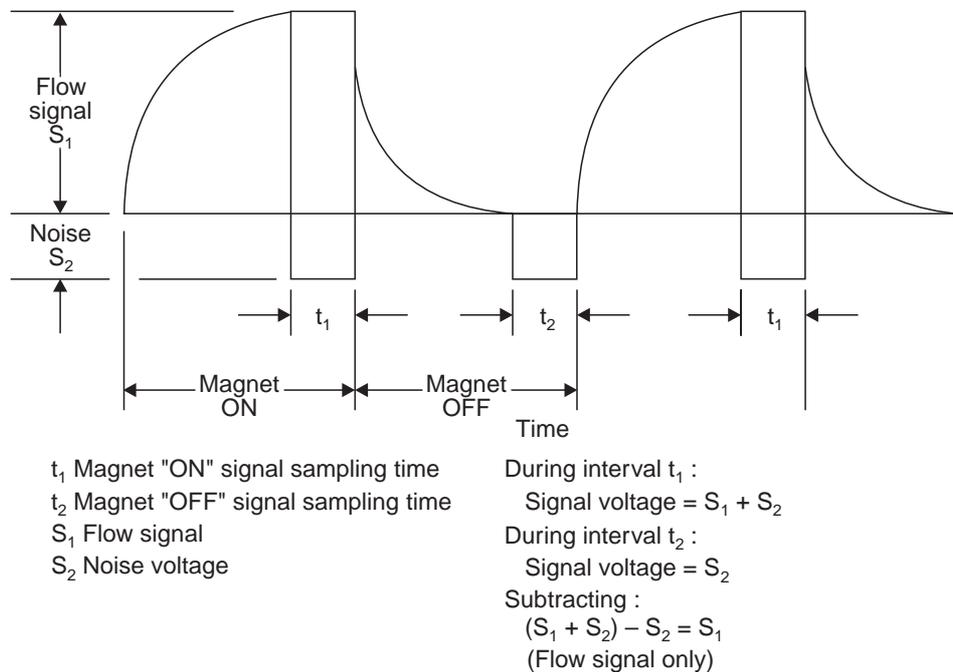
Fig. 1.54 Plot of the output signal
