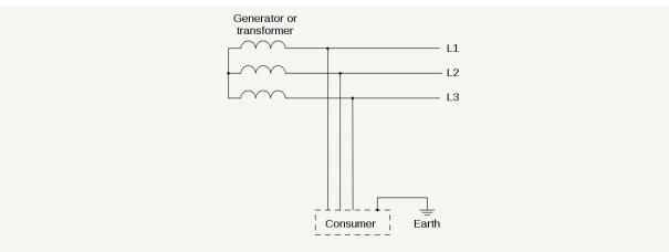
With IT earthing system, the power supply has no point connected with earth (source: Wikipedia)
