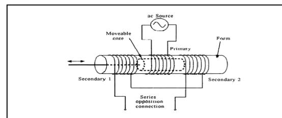
Figure 2. LVDT schematic diagram
