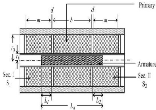
Figure. 3 Cross-section of LVDT
