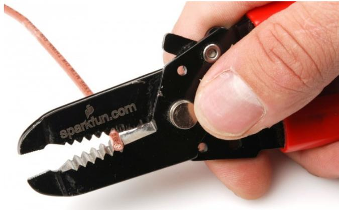
By simply squeezing the handles about  $\frac{1}{4}$ " from the end of the wire or the desired length, using the correct notch on the tool, and then twisting it slightly, the insulation will be cut free.
