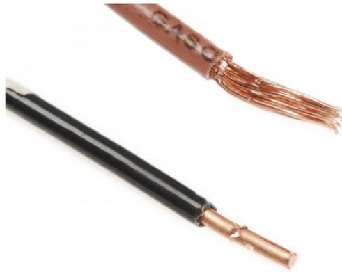
*This wire was not stripped properly, there are gouges and missing strands*
