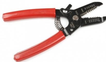
A simple manual wire stripper is a pair of opposing blades much like scissors. There are several notches of varying size. This allows the user to match the notch size to the wire size, which is very important for not damaging the wires.
