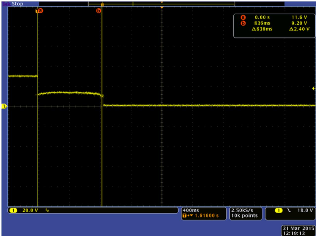
While the arc was in progress and intermediate current flows, implying the relay package has to dissipate significant power during the arc duration.
